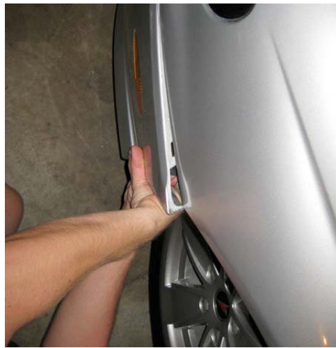
Figure 3. Rear of bumper free from fender
