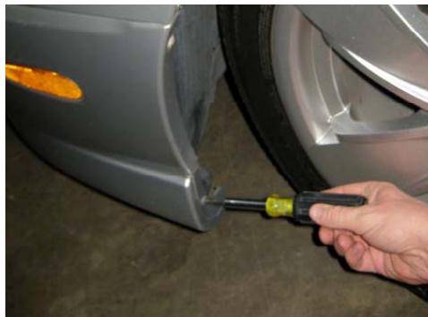
Figure 1. Remove screws with phillips screwdriver.
