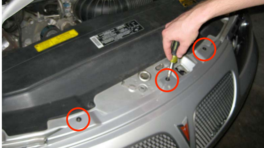
Figure 6. Screws are circled in red.
