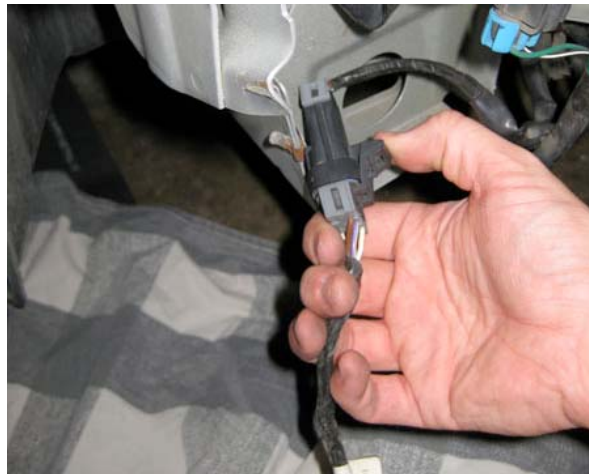
Figure 7. Release the wiring connector for the foglights.
